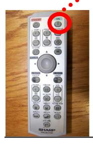
Point this remote at the projector hanging from the ceiling and press the "ON" button. You should hear the fan come on. It will take a minute or two for the unit to warm up.
