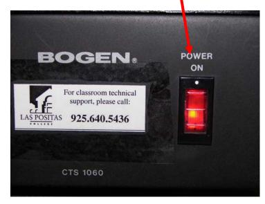
Turn on the audio amplifier unit located in the closet - the orange light will glow.
